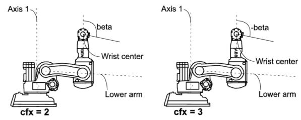
The following figure shows an example of robot configuration 4 and 5. Note the different signs of the axis 5 angle.
