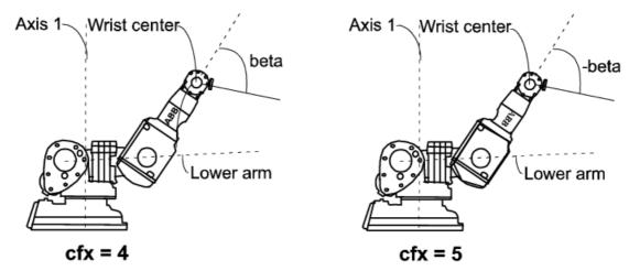
The following figure shows an example of robot configuration 6 and 7. Note the different signs of the axis 5 angle.
