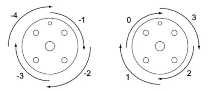
For a linear axis, the value defines a meter interval for the robot axis. For each axis, value 0 means a position between 0 and 1 meters and 1 means a position between 1 and 2 meters. For negative values, -1 means a position between -1 and 0 meters, and so on. The figure shows configuration values for a linear axis.
