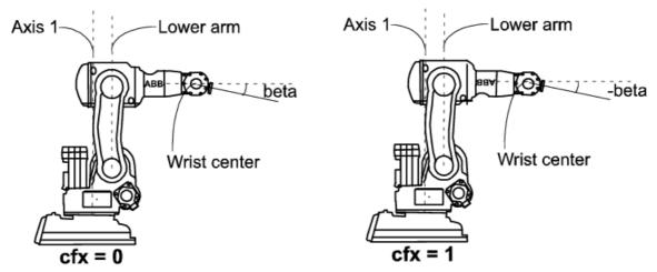
The following figure shows an example of robot configuration 2 and 3. Note the different signs of the axis 5 angle.
